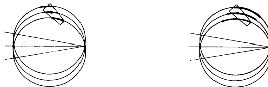
Fig. 15. Role of receiving aperture in scan of isolated reflection. Representation at left is for 2:1 scanning technique and representation at right is for \omega scan.
